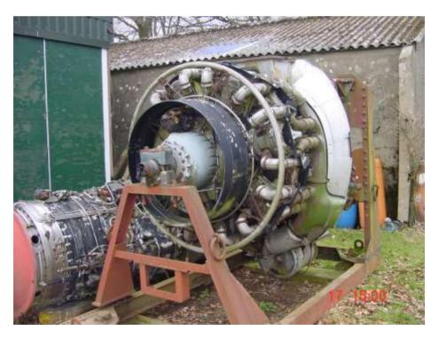
It is in fact an old sleeve valve radial engine; a Bristol Siddley Hercules 14 cylinder radial aircraft engine. (I must add immediately, I do not own it, nor do I know precisely who owns it, but I know it needs working on).
